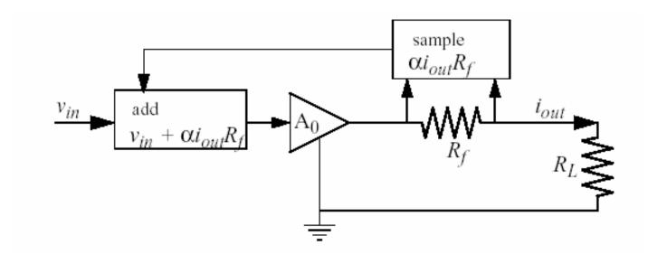
$$i_{out} = \frac{A_0 v_{in}}{R_L + Z_{out0} + (1 - A_0 \alpha) R_f}$$
