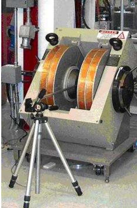
Fig. 5c. Scintillator Assembly between the magnet poles.
